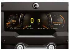
DIGITAL GAUGE Large panoramic 7.8" wide LCD color display with BRP Connect<sup>™</sup>, allowing the integration of vehicle-optimized smartphone apps such as media, navigation and many others controlled through the handlebars.
